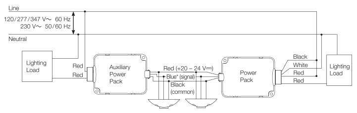
NOTE: Maximum of 3 devices total (occupancy sensors and auxiliary power packs) can be connected to a power pack.
